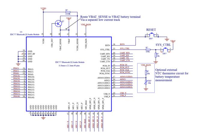
VDD\_PADS should be supplied by an external fixed voltage regulator in this configuration to provide a constant voltage reference for the IO supply domain. When connected to a battery a buck/boost synchronous regulator is recommended, the circuit below provides an example.
