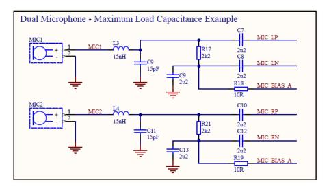
If a single microphone is used, the unused analogue inputs should be AC coupled to ground.
